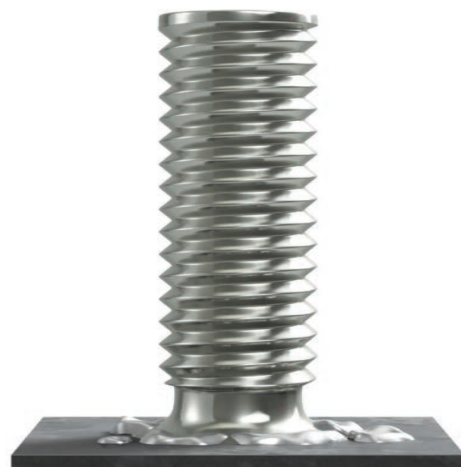
f. Stud weld made with excessive heat
