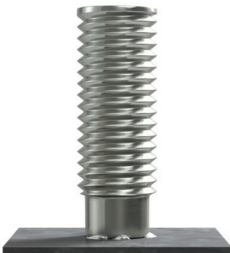
e. Stud weld made with insufficient heat
