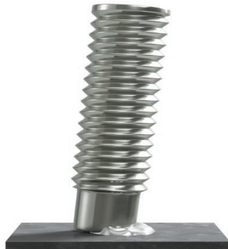
d. Poor alignment
